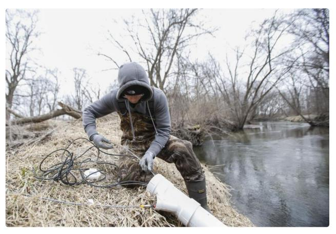
Jason McCurdy, a researcher and field technician at the IIHR Hydroscience and Engineering center at the University of lowa's College of Engineering, in 2017 installs a water quality sensor used for testing nitrate levels at Miller Creek, west of Gilbertville. The program has installed the sensors across the state in order to establish a baseline report of various water quality indicators. (The Gazette)
